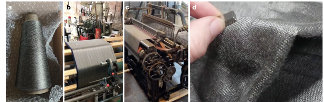
Figure 3: a) Custom ferromagnetic yarns that were integrated through b-c) weaving process to create d) magnetic textiles.
