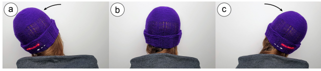
Figure 18: Hands-free turn signals for cyclists - made with an LED fiber controlled by the MCU and the accelerometer.
