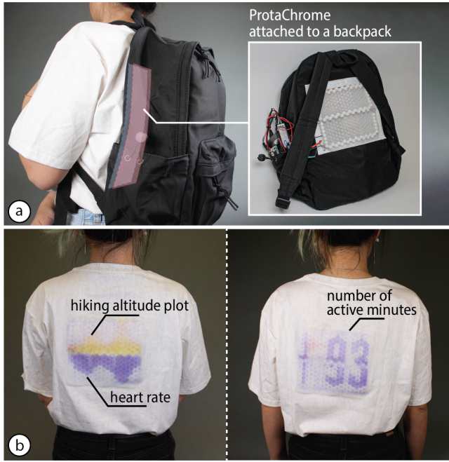
Figure 14: PortaChrome can be attached to a backpack and create customized patterns on the back of a user's T-shirt. (a) PortaChrome is sewed onto a backpack powered with a battery pack. (b) PortaChrome reprograms the back of the T-shirt to visualize the user's hiking trail and heart rate, and displays the number of active minutes spent on this hike.
