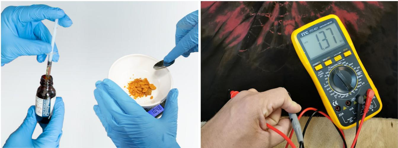
**Figure 3: The chemical products used to functionalize our textile, Pyrrole and Iron Chloride (left). After functionalization, the textile is conductive, except where it was tied (right).**
