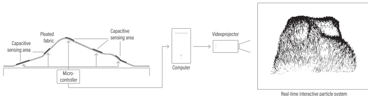
Figure 2: System Summary: sensing structure (left), computing and projection (right)
