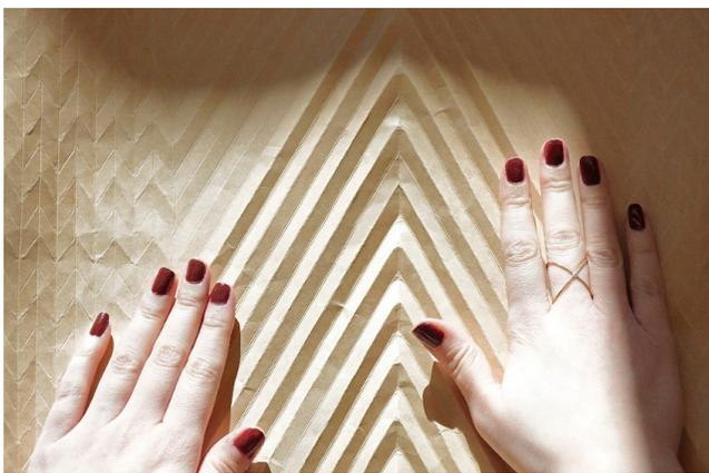
**Figure 4: This cardboard mold is used to create the Peacock Pattern (credit: Anne Combaz, Ateliers Lognon).**
