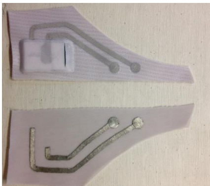
Figure 4 - eTextile battery pouch detail
