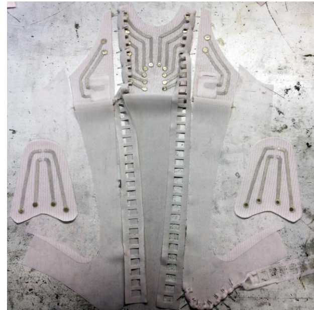
Figure 5 Toile #2: Second Skin pattern piece layout showing assembled eTextile panels and laser cut ladders to house tubing for cables
