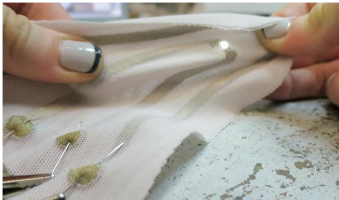
Figure 1: Testing the elasticity of a stretch circuit panel. The LED and button are inserted into tiny unbonded pockets, through tiny slits the back of the fabric, and secured with conductive thread. Please refer to our video figure to see the sample being stretched.
