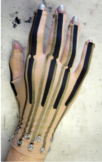
Figure 7- Fabric concept for eTextile mi.mu glove ( http://mimugloves.com/ ) which inspired the second skin project (2015)
