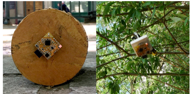
Figure 2. The Twiz motion sensor mounted onto a Motion Sensing Extension (left), and attached to the branch of a tree to capture the movement of the wind swaying through the leaves (right).
