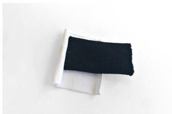
Figure 3: Non polymerized (white) and polymerized (black) samples
